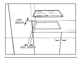
Because of the heat given off, there must be a minimum distance as follows:
